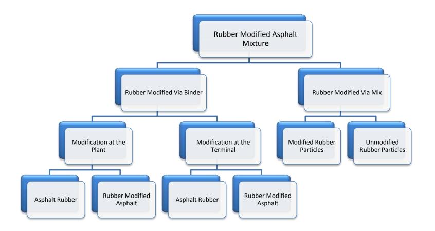
Asphalt Mix Modified via Binder (GTR added to binder) or via Mix (GTR added to aggregate during the mixing process)
